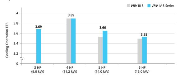
$\star$ Cooling operation conditions: Indoor temp. of 27° CDB,19° CWB, and outdoor temp. of 35° CDB
