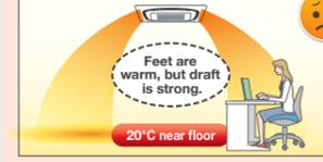
Uncomfortable draft occurs, because air is blown downward. To avoid draft, air direction is changed to horizontal and feet get cold.
