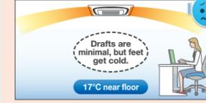
Feet get cold, because warm air collects near the ceiling. Area near floor doesn't reach set temperature and feet feel cold. For this reason, we end up raising the temperature setting.
