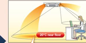
In order to reduce drafts, air is blown horizontally where a person is located.\*9
