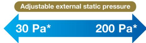
Set to low static pressure when ducts are short.
