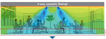
Width 7.5m x depth 7.5m x height 2.6m ■ Indoor unit capacity:71 class Outdoor air temperature:35°C
