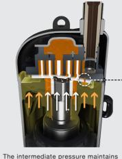
pressure on the orbiting scroll during low-load operation.
