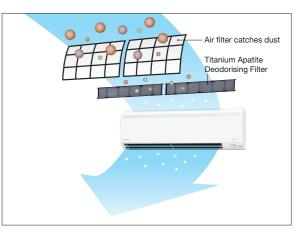
This filter is not a medical device. Benefits such as the adsorption of odours and allergens and deodorisation of odours are only effective for substances which are directly attached to the Titanium Apatite Deodorising Filter.
