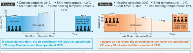
Shift temperature and time can be selected from 0.5 to 4°C in 0.5°C increments and 15, 30, 45, 60, 90 or 120 minutes respectively with remote controller.
