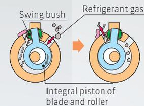
The swing compressor can reduce operational vibration and sound because its piston moves smoothly inside the compressor.
