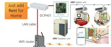
\*A separate power supply for Home Automation Interface Adaptor is necessary. It may not be installed inside some outdoor unit models.
