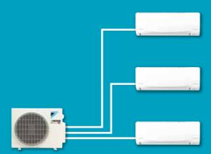
With multi-split systems, a single outdoor unit can easily power several indoor units. Three rooms only require one outdoor unit.
