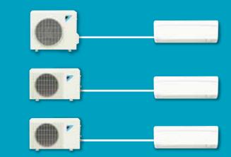
With split type air conditioners, you need one outdoor unit for every indoor unit. Three rooms mean three outdoor units.
