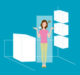
If three outdoor units are installed on a balcony, the workspace is too narrow.
