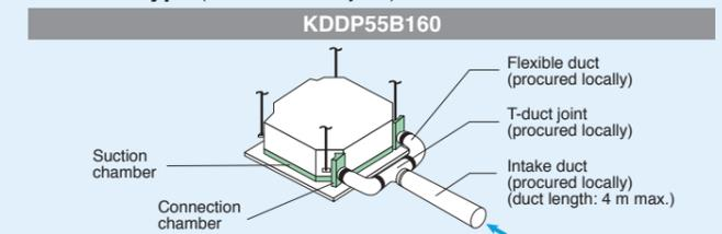
**Chamber type (with T-duct joint)** Note 3.4
