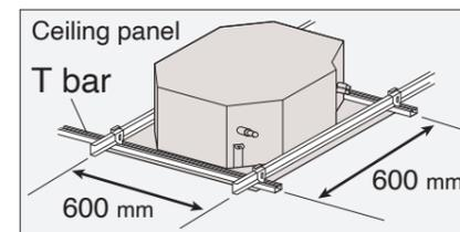
The control box is built in to the unit, so maintenance is possible by simply removing the grille. An inspection opening is not required even for modules other than 600 x 600.
