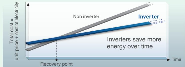
Inverter air conditioner can adjust its cooling capacity according to the cooling load. This results in less power consumption.
