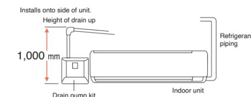
Drain pump kit can be installed on either left and right side of the indoor unit.
