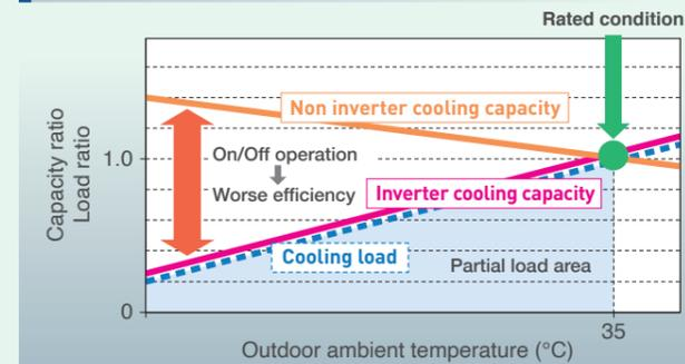
In response to fluctuating cooling load, non-inverter air conditioners repeatedly perform On (full-power)/Off (zero-power) operation. Inverter air conditioners, however, operate at optimal cooling capacity according to the cooling load. Since inverter air conditioners provide required minimum cooling capacity with minimum electrical power, total power consumption can be reduced during cooling period.
