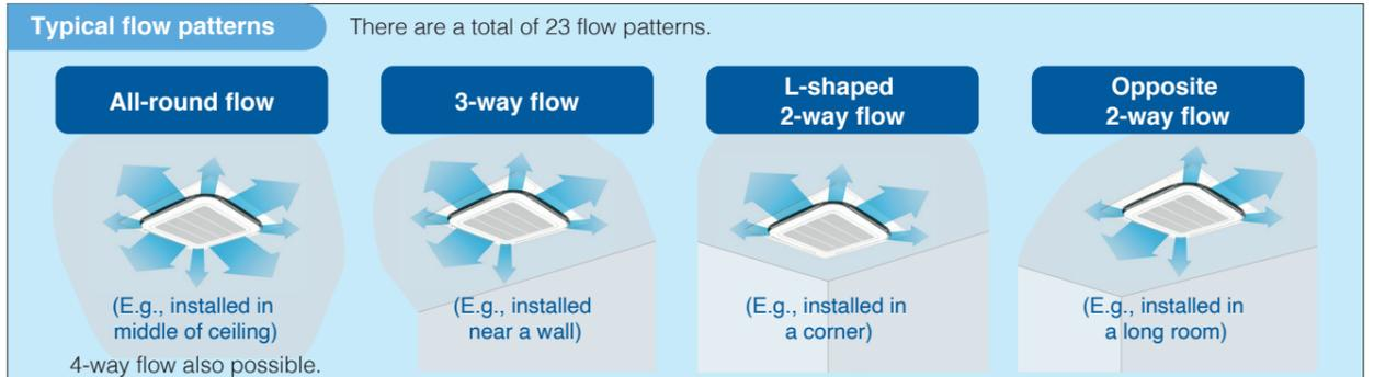
Note: Whatever the discharge direction, the same type of panel is used. If installing for other than all-round flow, an air discharge outlet sealing material (option) must be used to close each unused outlet. Operation sound increases when using 2-way or 3-way flow.
