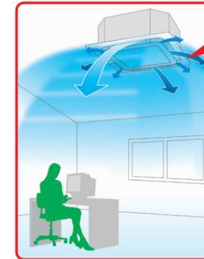
360° airflow can maintain comfort even if air discharge speed is lower.
